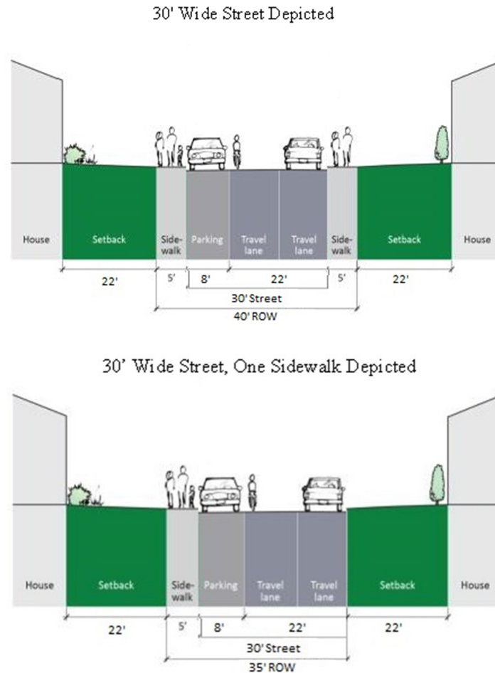
Figure 10.24.120(b)(2) (Continued) Cross-sections for local access street design options (with standard dimensions).
